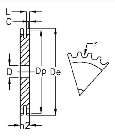
C = 1 D = 20 De = 368.3 Dp = 363.86 For chain size =  $3/8 \times 7/32$ For chain type = 06 B-2 h2 = 5.3
